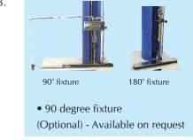
Peel Strength Tester reveals the peeling strength force required to remove pressure sensitive coated material, which has been applied to standard test specimen under specified conditions from the plate at a specified angle and speed.
